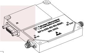
PIN **DESCRIPTION** +28V 1 2 +28V 3 **GND** 4 **GND** N/C 5 N/C 6 **OVER-CURRENT BIT** 7 8 **BLANKING TTL** 9 +28V +28V 10 GND 11 12 **GND** 13 N/C 14 N/C **OVER-TEMP BIT**
