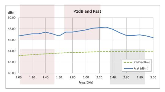
50 dB Gain High Power GaN Amplifier at 50 Watt Psat Operating from 1 GHz to 3 GHz with SMA from Fairview Microwave is in-stock and available to ship same-day. All of our RF/microwave products are available off-the-shelf from our ISO 9001:2008 certified facilities in Allen, Texas. Fairview Microwave is RF on-demand.
