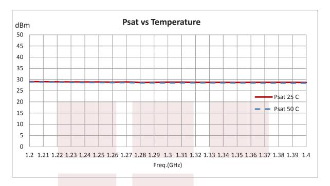
46 dB Gain Medium Power High Gain Amplifier at 600 mW Psat Operating From 1.2 GHz to 1.4 GHz with SMA from Fairview Microwave is in-stock and available to ship same-day. All of our RF/microwave products are available off-the-shelf from our ISO 9001:2008 certified facilities in Allen, Texas. Fairview Microwave is RF on-demand.
