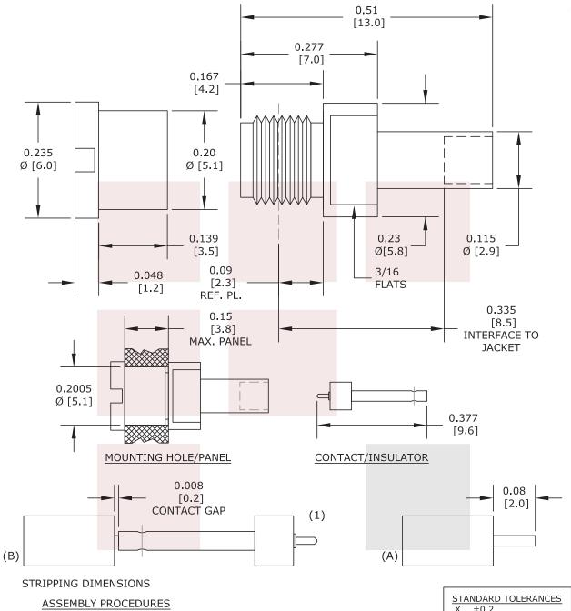
1. STRIP CABLE AS SHOWN IN (A). DO NOT NICK CENTER CONDUCTOR.
