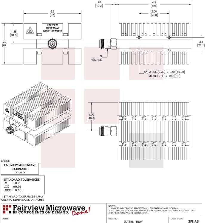
RF Load 100 Watts High Power To 8 GHz Conduction Cooled Body Black Anodized Aluminum Heatsink N Female
