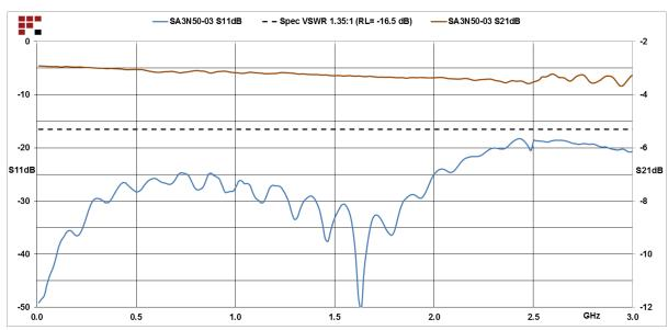
3 dB Fixed Attenuator N Male (Plug) to N Female (Jack) Up to 3 GHz Rated to 50 Watts, Heatsink Body, 1.35 VSWR from Fairview Microwave is in-stock and available to ship same-day. All of our RF/microwave products are available off-the-shelf from our ISO 9001:2008 certified facilities in Lewisville, Texas. Fairview Microwave is RF on-demand.
