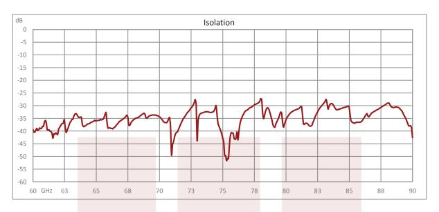
WR-12 Waveguide Isolator with 25 dB min Isolation from 60 GHz to 90 GHz using Round Cover UG-387/U Flange from Fairview Microwave is in-stock and available to ship same-day. All of our RF/microwave products are available off-the-shelf from our ISO 9001:2008 certified facilities in Allen, Texas. Fairview Microwave is RF on-demand.
