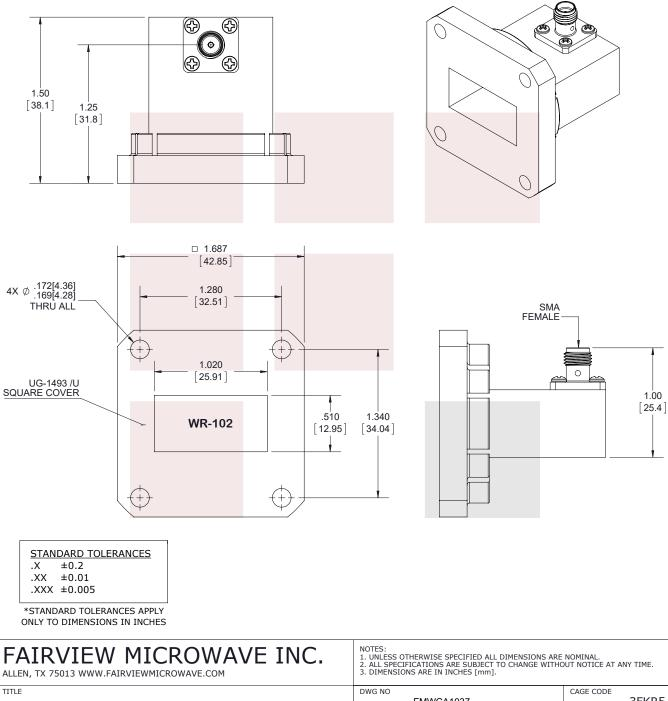
WR-102 to SMA Female Waveguide to Coax Adapter UG-1493/U Square Cover with 7 GHz to 10 GHz in Aluminum, Paint
