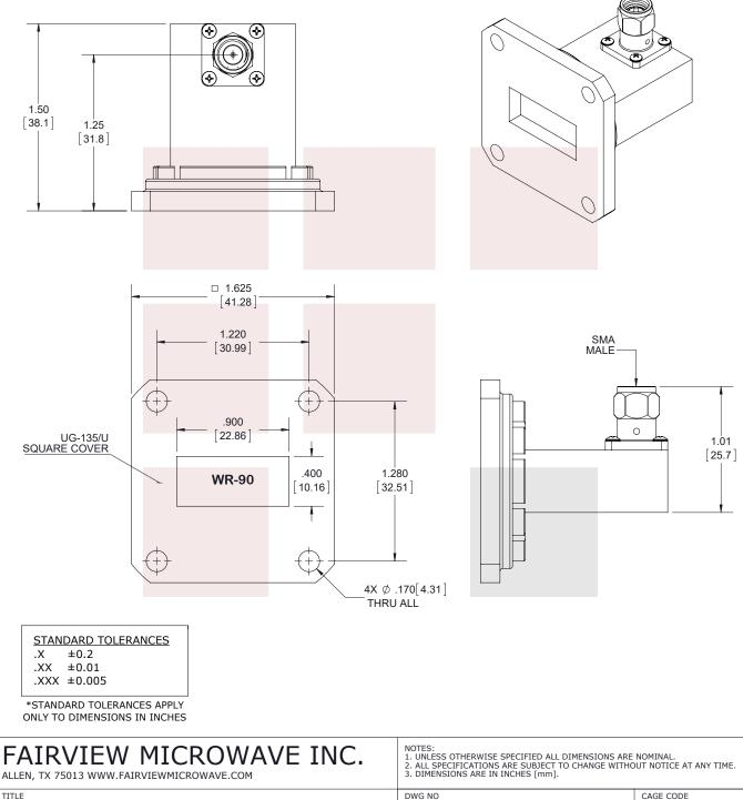
WR-90 to SMA Male Waveguide to Coax Adapter UG-135/U Square Cover with 8.2 GHz to 12.4 GHz X Band in Aluminum, Paint
