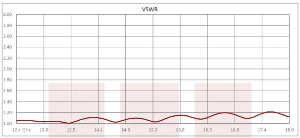
WR-62 to Type N Female Waveguide to Coax Adapter UG-1665/U Square Cover with 12.4 GHz to 18 GHz Ku Band in Aluminum, Paint from Fairview Microwave is in-stock and available to ship same-day. All of our RF/microwave products are available off-the-shelf from our ISO 9001:2008 certified facilities in Lewisville, Texas. Fairview Microwave is RF on-demand.
