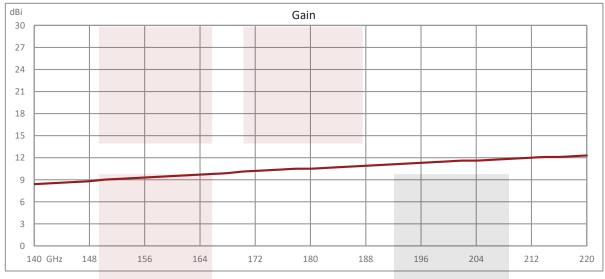
Conical Gain Horn Waveguide Antenna, WR-5, 140 GHz to 220 GHz, UG-387/U Round Cover Flange, 10 dBi Nominal Gain from Fairview Microwave is in-stock and available to ship same-day. All of our RF/microwave products are available off-the-shelf from our ISO 9001:2008 certified facilities in Allen, Texas. Fairview Microwave is RF on-demand.
