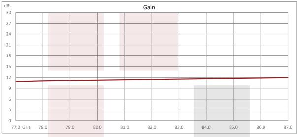
Conical Gain Horn Waveguide Antenna, WR-12, 77 GHz to 87 GHz, UG-387/U Round Cover Flange, 10 dBi Nominal Gain from Fairview Microwave is in-stock and available to ship same-day. All of our RF/microwave products are available off-the-shelf from our ISO 9001:2008 certified facilities in Allen, Texas. Fairview Microwave is RF on-demand.
