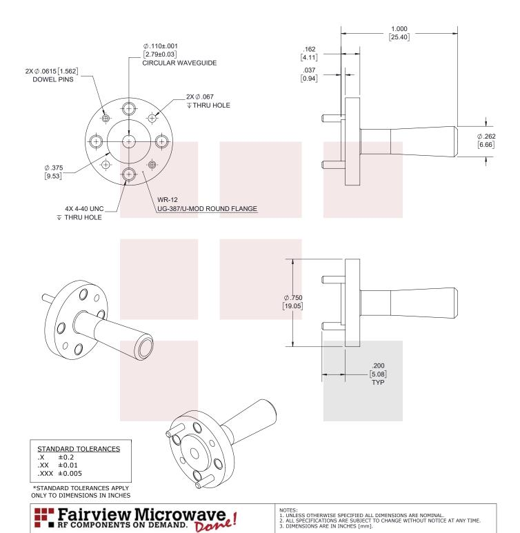
Conical Gain Horn Waveguide Antenna, WR-12, 77 GHz to 87 GHz, UG-387/U Round Cover Flange, 10 dBi
