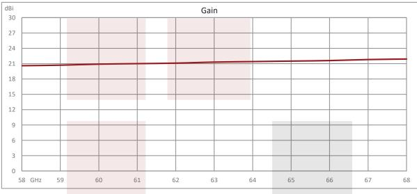
Conical Gain Horn Waveguide Antenna, WR-15, 58 GHz to 68 GHz, UG-385/U Round Cover Flange, 20 dBi Nominal Gain from Fairview Microwave is in-stock and available to ship same-day. All of our RF/microwave products are available off-the-shelf from our ISO 9001:2008 certified facilities in Allen, Texas. Fairview Microwave is RF on-demand.
