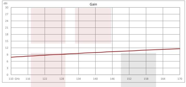
Standard Gain Horn Waveguide Antenna, WR-6, 110 GHz to 170 GHz, UG-387/U-Mod Round Cover Flange, 10 dBi Nominal Gain from Fairview Microwave is in-stock and available to ship same-day. All of our RF/microwave products are available off-the-shelf from our ISO 9001:2008 certified facilities in Allen, Texas. Fairview Microwave is RF on-demand.
