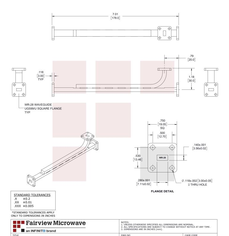
20 dB WR-28 Waveguide Broadwall Coupler with UG-599/U Square Cover Flange and E-Plane Coupled Port
