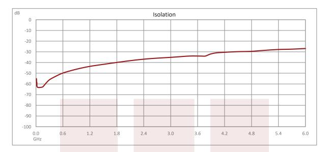
SMA Reflective SPDT GaN High Power PIN Diode Switch from DC to 6 GHz Rated at 40 Watts < 100ns Speed with Heatsink from Fairview Microwave is in-stock and available to ship same-day. All of our RF/microwave products are available off-the-shelf from our ISO 9001:2008 certified facilities in Lewisville, Texas. Fairview Microwave is RF on-demand.
