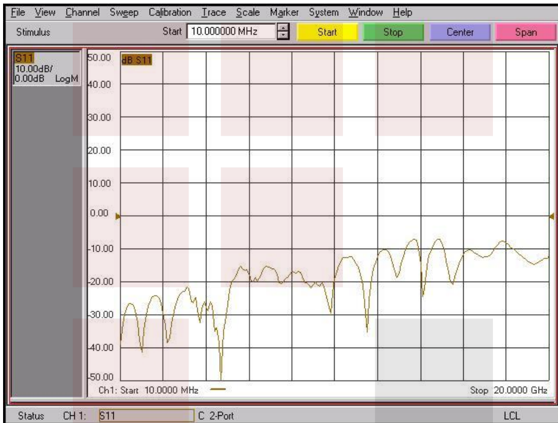
TEST DATA TAKEN WITH 2 FMPB1002 PROBES (IN/OUT) ON EITHER END OF A 40mm COPLANAR WAVEGUIDE
