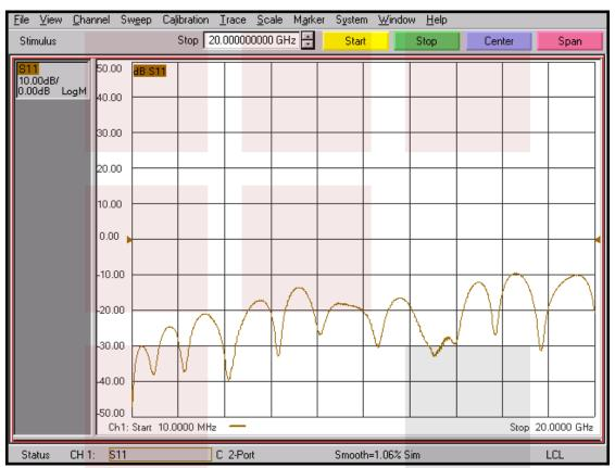
TEST DATA TAKEN WITH 2 FMPB1001 PROBES (IN/OUT)
