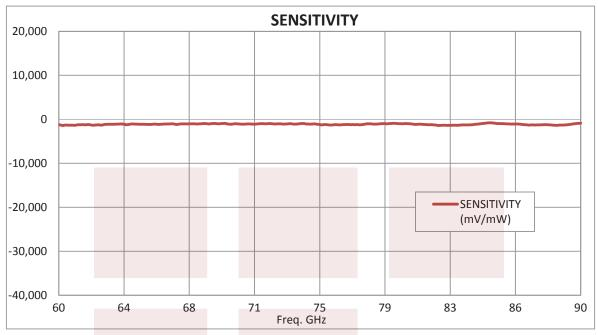
Zero Biased Waveguide Detector WR-12 to SMA Female and Negative Video Out From 60 GHz to 90 GHz E Band, UG-387/U Round Cover Flange from Fairview Microwave is in-stock and available to ship same-day. All of our RF/microwave products are available off-the-shelf from our ISO 9001:2008 certified facilities in Allen, Texas. Fairview Microwave is RF on-demand.
