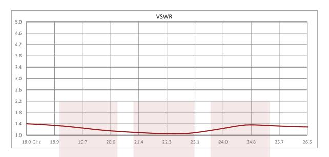
Isolator 2.92mm Female, Hermetically Sealed with 14 dB Isolation from 18 GHz to 26.5 GHz Rated to 10 Watts from Fairview Microwave is in-stock and available to ship same-day. All of our RF/microwave products are available off-the-shelf from our ISO 9001:2008 certified facilities in Lewisville, Texas. Fairview Microwave is RF on-demand.
