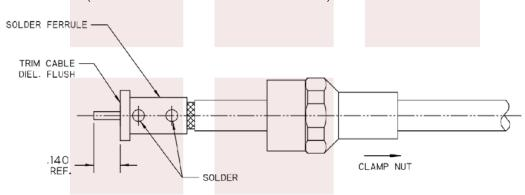
3. SOLDER CONTACT WITH GAP INDICATED AS SHOWN.
