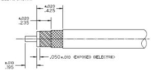
2. INSERT CABLE INTO SOLDER FERRULE UNTIL BRAIDS SEAT IN FERRULE. THEN SOLDER BOTH CABLE BRAIDS TO FERRULE WHERE SHOWN. TRIM CABLE DIELECTRIC FLUSH WITH FACE OF FERRULE.
