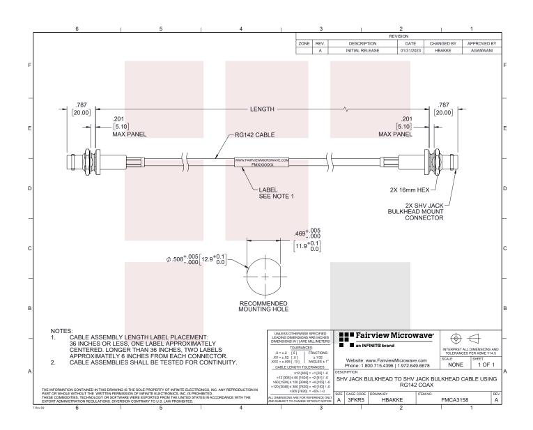
SHV Jack Bulkhead to SHV Jack Bulkhead Cable RG-142 Coax
