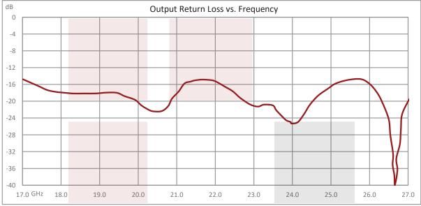
Negative Slope Equalizer, 18 GHz to 26 GHz, 6 dB Fixed Equalizing Value, 1.3 dB Loss, Max Pin 250 mW, SMA from Pasternack Enterprises has same day shipment for domestic and International orders Our RF, microwave and millimeter wave products maintain a 99.4% availability and are part of the broadest selection in the industry.
