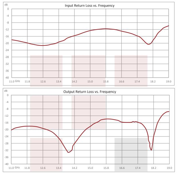
Negative Slope Equalizer, 12 GHz to 18 GHz, 7 dB Fixed Equalizing Value, 0.65 dB Loss, Max Pin 150 mW, SMA from Pasternack Enterprises has same day shipment for domestic and International orders Our RF, microwave and millimeter wave products maintain a 99.4% availability and are part of the broadest selection in the industry.
