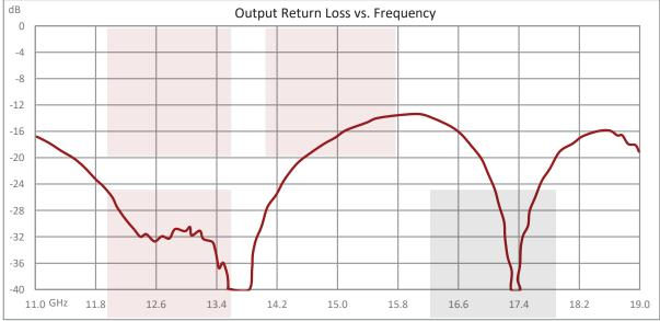
Negative Slope Equalizer, 12 GHz to 18 GHz, 3 dB Fixed Equalizing Value, 0.9 dB Loss, Max Pin 150 mW, SMA from Pasternack Enterprises has same day shipment for domestic and International orders Our RF, microwave and millimeter wave products maintain a 99.4% availability and are part of the broadest selection in the industry.
