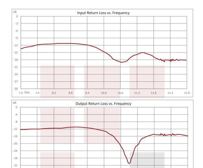
Negative Slope Equalizer, 8 GHz to 12 GHz, 10 dB Fixed Equalizing Value, 0.6 dB Loss, Max Pin 250 mW, SMA from Pasternack Enterprises has same day shipment for domestic and International orders Our RF, microwave and millimeter wave products maintain a 99.4% availability and are part of the broadest selection in the industry.
