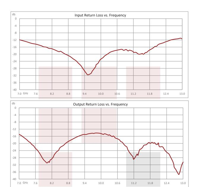
Negative Slope Equalizer, 8 GHz to 12 GHz, 3 dB Fixed Equalizing Value, 0.3 dB Loss, Max Pin 250 mW, SMA from Pasternack Enterprises has same day shipment for domestic and International orders Our RF, microwave and millimeter wave products maintain a 99.4% availability and are part of the broadest selection in the industry.
