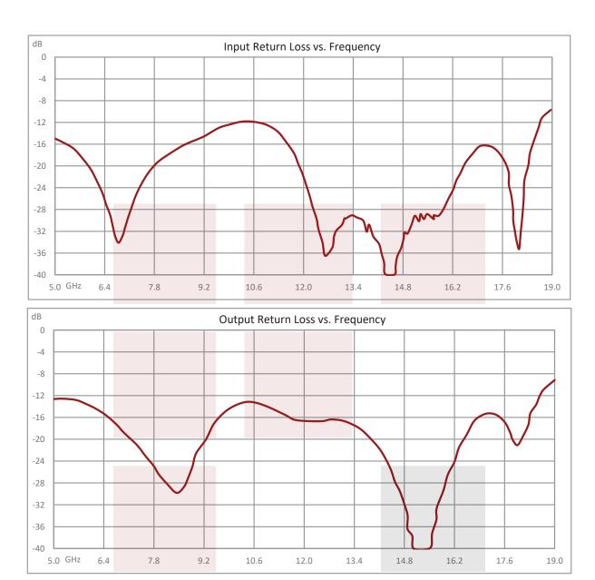
Negative Slope Equalizer, 6 GHz to 18 GHz, 3 dB Fixed Equalizing Value, 0.9 dB Loss, Max Pin 150 mW, SMA from Pasternack Enterprises has same day shipment for domestic and International orders Our RF, microwave and millimeter wave products maintain a 99.4% availability and are part of the broadest selection in the industry.
