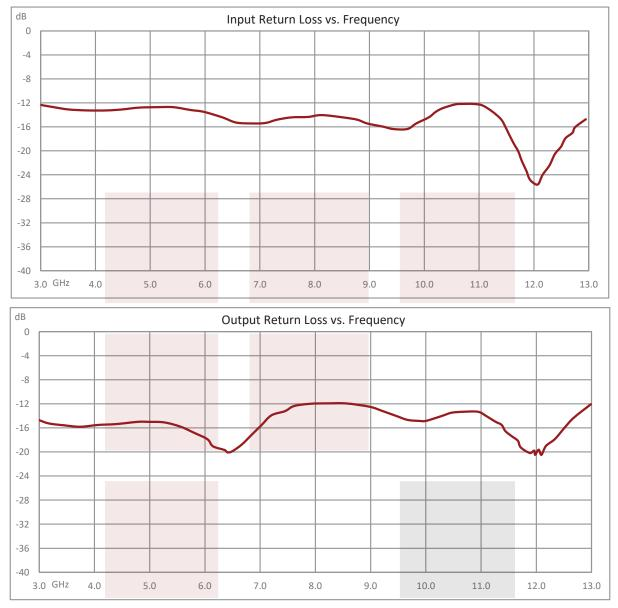
Negative Slope Equalizer, 4 GHz to 12 GHz, 9 dB Fixed Equalizing Value, 0.3 dB Loss, Max Pin 250 mW, SMA from Pasternack Enterprises has same day shipment for domestic and International orders Our RF, microwave and millimeter wave products maintain a 99.4% availability and are part of the broadest selection in the industry.
