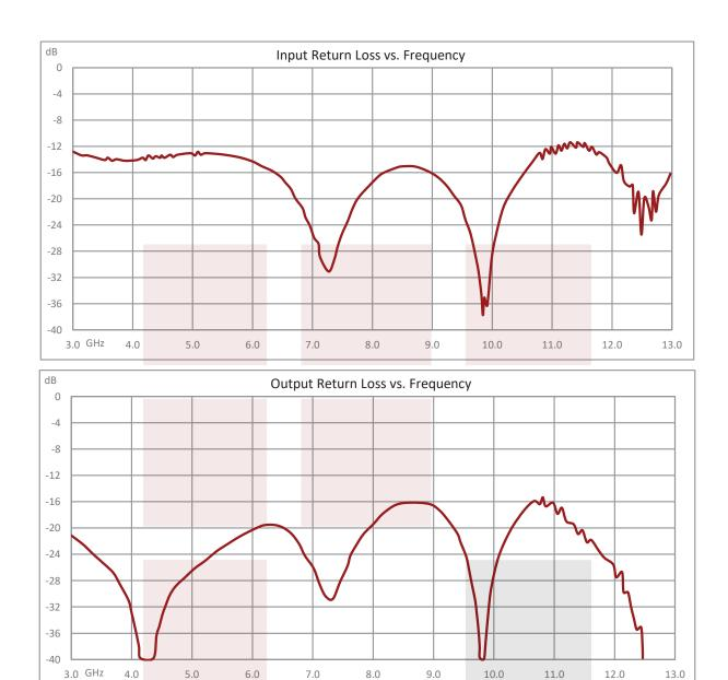
Negative Slope Equalizer, 4 GHz to 12 GHz, 6 dB Fixed Equalizing Value, 0.5 dB Loss, Max Pin 250 mW, SMA from Pasternack Enterprises has same day shipment for domestic and International orders Our RF, microwave and millimeter wave products maintain a 99.4% availability and are part of the broadest selection in the industry.
