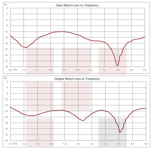
Negative Slope Equalizer, 4 GHz to 8 GHz, 6 dB Fixed Equalizing Value, 0.6 dB Loss, Max Pin 250 mW, SMA from Pasternack Enterprises has same day shipment for domestic and International orders Our RF, microwave and millimeter wave products maintain a 99.4% availability and are part of the broadest selection in the industry.
