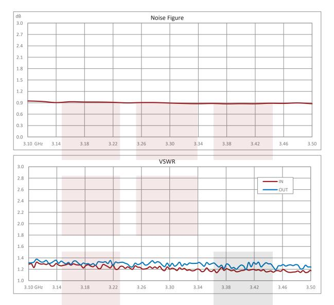
0.8 dB NF Input Protected Low Noise Amplifier, Operating from 3.1 GHz to 3.5 GHz with 28 dB Gain, 8 dBm P1dB and SMA from Fairview Microwave is in-stock and available to ship same-day. All of our RF/microwave products are available off-the-shelf from our ISO 9001:2008 certified facilities in Allen, Texas. Fairview Microwave is RF on-demand.
