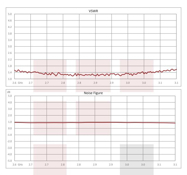
1.2 dB NF Input Protected Low Noise Amplifier, Operating from 2.6 GHz to 3.1 GHz with 40 dB Gain, 10 dBm P1dB and SMA from Fairview Microwave is in-stock and available to ship same-day. All of our RF/microwave products are available off-the-shelf from our ISO 9001:2008 certified facilities in Allen, Texas. Fairview Microwave is RF on-demand.
