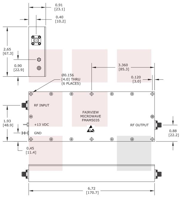
NOTE: HEAT SINK REQUIRED FOR PROPER OPERATION, UNIT IS COOLED BY CONDUCTING TO HEAT SINK.
