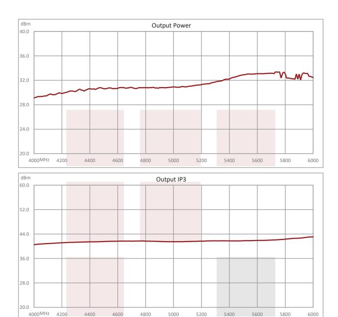
1 Watt P1dB, 4 GHz to 6 GHz, Medium Power GaAs Amplifier, 30 dB Gain, 42 dBm IP3 and SMA from Fairview Microwave is instock and available to ship same-day. All of our RF/microwave products are available off-the-shelf from our ISO 9001:2008 certified facilities in Lewisville, Texas. Fairview Microwave is RF on-demand.
