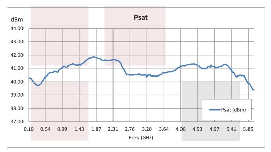
60 dB Gain High Power Amplifier at 10 Watt Psat Operating from 100 MHz to 6 GHz with SMA Input, SMA Output from Fairview Microwave is in-stock and available to ship same-day. All of our RF/microwave products are available off-the-shelf from our ISO 9001:2008 certified facilities in Allen, Texas. Fairview Microwave is RF on-demand.
