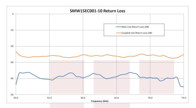
WR-15 Directional Waveguide Coupler 10 dB With UG-385/U Flange and E-Plane Coupled Port From 50 GHz to 75 GHz V Band from Fairview Microwave is in-stock and available to ship same-day. All of our RF/microwave products are available off-the-shelf from our ISO 9001:2008 certified facilities in Allen, Texas. Fairview Microwave is RF on-demand.
