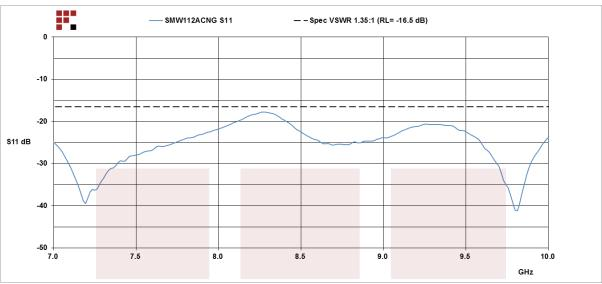
WR-112 to N Female Waveguide to Coax Adapter PDR84 Flange With 7.05 GHz to 10 GHz Frequency Range For X Band from Fairview Microwave is in-stock and available to ship same-day. All of our RF/microwave products are available off-the-shelf from our ISO 9001:2008 certified facilities in Allen, Texas. Fairview Microwave is RF on-demand.
