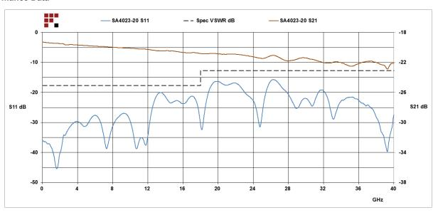
20 dB Fixed Attenuator 2.92mm Male (Plug) to 2.92mm Female (Jack) Directional Up to 40 GHz Rated to 20 Watts, Heatsink Body, 1.4 VSWR from Fairview Microwave is in-stock and available to ship same-day. All of our RF/microwave products are available off-the-shelf from our ISO 9001:2008 certified facilities in Lewisville, Texas. Fairview Microwave is RF on-demand.
