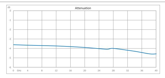
4 dB Fixed Attenuator 2.92mm Male (Plug) to 2.92mm Female (Jack) Up to 40 GHz Rated to 1 Watt, Passivated Stainless Steel Body, 1.4 VSWR from Fairview Microwave is in-stock and available to ship same-day. All of our RF/microwave products are available off-the-shelf from our ISO 9001:2008 certified facilities in Lewisville, Texas. Fairview Microwave is RF on-demand.
