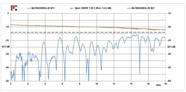
20 dB Fixed Attenuator N Male (Plug) to N Female (Jack) Directional Up to 18 GHz Rated to 200 Watts, Heatsink Body, 1.5 VSWR from Fairview Microwave is in-stock and available to ship same-day. All of our RF/microwave products are available off-the-shelf from our ISO 9001:2008 certified facilities in Lewisville, Texas. Fairview Microwave is RF on-demand.
