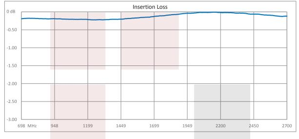
4 Way High Power Equal Tapper with 4.1/9.5 Mini DIN Operating from 600 MHz to 2.7 GHz Rated at 300 Watts from Fairview Microwave is in-stock and available to ship same-day. All of our RF/microwave products are available off-the-shelf from our ISO 9001:2008 certified facilities in Allen, Texas. Fairview Microwave is RF on-demand.
