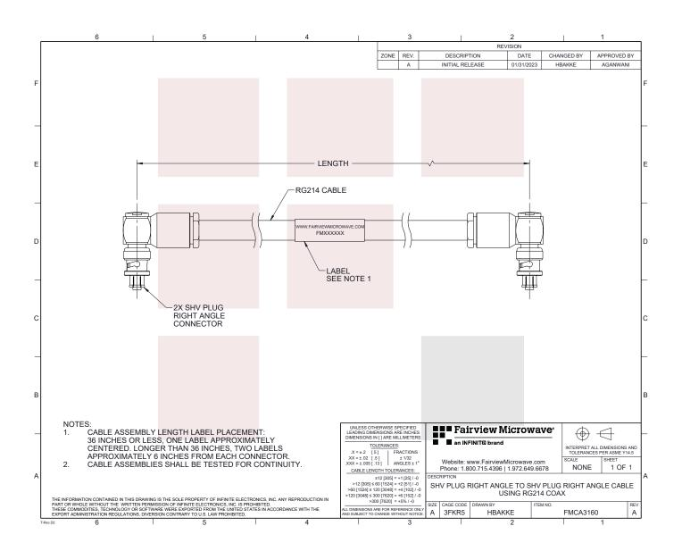
RA SHV Plug to RA SHV Plug Cable RG-214 Coax in 48 Inch
