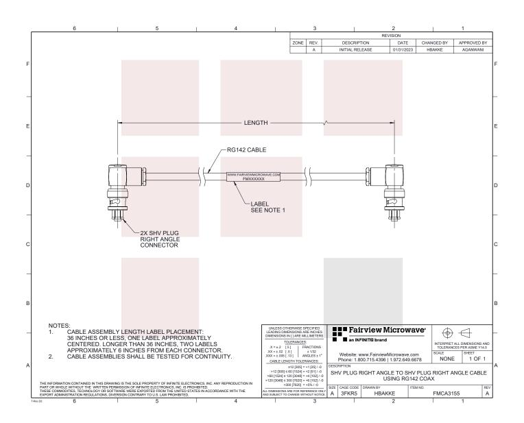
RA SHV Plug to RA SHV Plug Cable RG-142 Coax in 36 Inch
