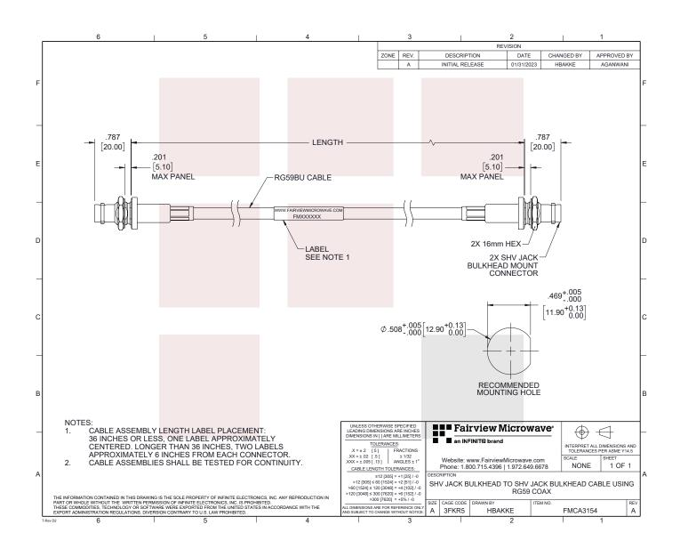
SHV Jack Bulkhead to SHV Jack Bulkhead Cable 75 Ohm RG59 Black Coax in 36 Inch
