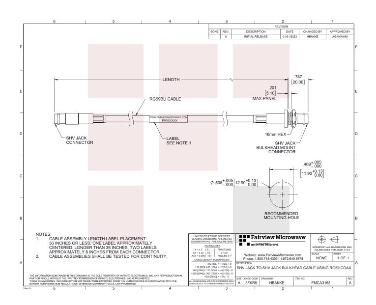
SHV Jack to SHV Jack Bulkhead Cable 75 Ohm RG-59 Black Coax in 60 Inch
