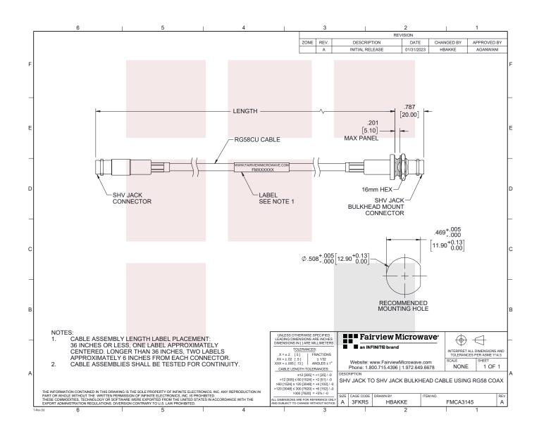
SHV Jack to SHV Jack Bulkhead Cable RG-58 Coax in 60 Inch
