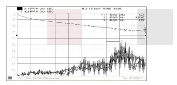
ELECTRICAL LENGTH (TWO WAY) = 5473PS ELECTRICAL LENGTH (ONE WAY) = 2736PS
