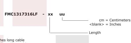
Example: FMC1317316LF-12 = 12 inches long cable FMC1317316LF-100cm = 100 cm long cable
