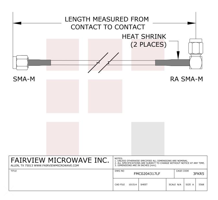
SMA Male to RA SMA Male Cable RG316-DS Coax in 24 Inch with LF Solder
